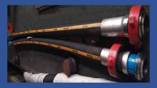
MUD KELLY HOSE OD:4" 75 FOOT FOOT LONG WITH CHAIN AND HAMMER UNION AND FITTINGS FLEXIBLE HOSE WITH API 7K PME RUBBER HIGH PRESSURE GRADE:F STRENGTH SPIRAL STEEL WIRE
