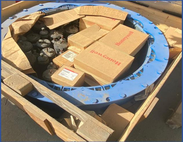
DISC BRAKES FOR DRAWWORKS HONEY WELL COMPANY PRESSURE:75KN THIKNESS :12MM,ELECTRIC STROKE :30 MMMATERIAL CLASS NON-ASBESTOS FRICTION
