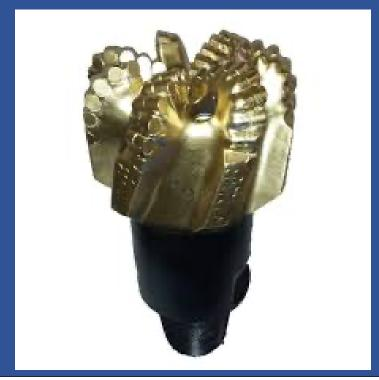
17-1/2 PDC BIT MATRIX BODY 6 BLADES CUTTRR 19 WITH 7-5/8 REGULAR PIN UP CONNECTION TYPE S236 WITH PORT MAXIMUM TOURQE MAKE UP 53.100 FT/LBS BIT SUB OD 8-1/2"
