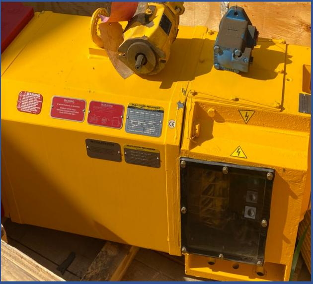
DRILL MAX 400-600 FOR TOP DRIVE VARCO(NATIONL OI-=[pL VALVE) MOTORS MODEL:TDS-11 SA BALDOR MANUFAACTURER COMPANY,HP:400,RPM:1155 AMP:366,PH:3,MAX SPEED 3750,AMB:50,SERIAL NO:B9150826,S.F:1.00 MATERIAL CLASS:STAINLESS STEEL CAST IRON
