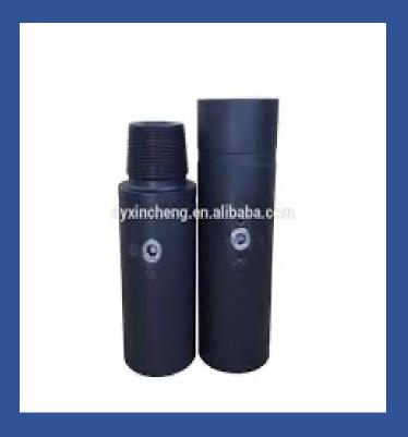
UPPER KELLY VALVE ,IBOP FOR VARCO TOP DRIVE FOR 5: DRILL PIPE WITH WRENCH LARGE BORE OD:6.34:,ID:2.750,LEGTH:28.60",PRESSURE RATING:10000 PSI CONNECTION:API 4-1/2" IF PIN&BOX MATERIAL CLASS:4145
